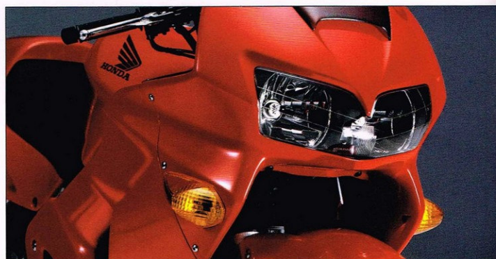
Side-mounted radiators improve cooling efficiency while the dual multi-reflector headlight's brilliant output is directed by the computer-designed angular reflectors.
