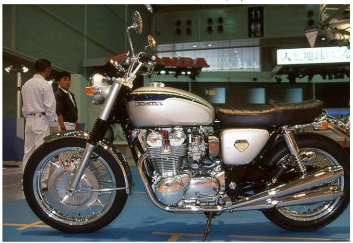
The 1999 <u>Honda CB750 F</u> was fitted with Dunlop TT100GP tyres in sizes 100/90-19 and 130/80-18, while the swingarm (which was covered by the two exhausts on each side) was made of steel tube. The two **rear shock absorbers** were also copied from those on the original bike, as were the chrome mudguards.
