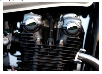
Not too far apart, not too close: the design team paid special attention to the positioning of the two camshafts. Freed from the necessity of maximizing output, they were able to establish the grand proportions that befit a large-displacement bike.
