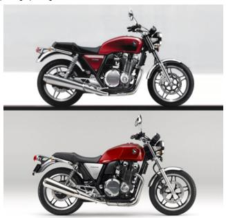
With just a few small changes, the silhouette can make a vastly different impression. An initial sketch version went all the way to the clay model stage. Finding it to be too tense, the designers went back to the drawing board. The difference between it and the final CB1100 is striking.
