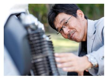
The cooling fins that cover the surface of the CB1100's air-cooled engine are quite different from the fins used to decorate a liquid-cooled engine, or the ribs used to strengthen one. Instead, they play the crucial role of increasing the surface area of the engine, thereby helping to disperse heat. At the same time, they give the naked engine a glorious appearance sure to draw admiring glances once the rider dismounts.
