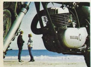
5-Port Engine Design: This is the Yamaha exclusive that still has the GP race crowds buzzing; a 5-port super scavenging system that gives the DT-1 an overall 10 percent increase in power and performance. Matched perfectly with a rugged 5-speed gearbox with gears spaced for sustained power under all trail and road conditions.
