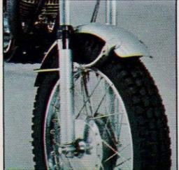
With no external springs and no rubber boots, Yamaha's rugged Enduro front forks are ready for all of the hard service you can give them in the roughest riding. And amazing comfort. Three-step rear suspension adjustable to meet every riding condition.
