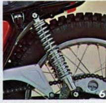
adjustable 6. Double-spring, rear shock absorbers. One spring smooths out the vibration caused by minor roughness in the road while the other spring cushions the larger shocks. The overall tension may be adjusted to any one of five positions according to the roughness of the road, and the type of riding.
