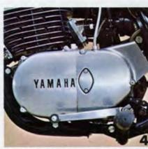
4. The constant-mesh, fully synchronized, 5-speed gearbox requires no break-in time. The shift lever is positioned for maximum operating ease, gently touch the lever with the tip of your foot and the transmission smoothly slides into gear. Yamaha 5-speeds give you the widest possible range for all types of ridina.
