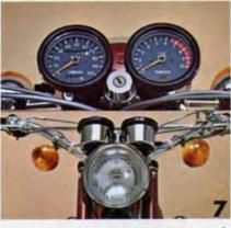
7. The precision tachometer and speedometer are designed for easy reading. The large, bright head lamp assures safe nighttime driving and the turn indicator lights are designed and mounted where they can be seen both day and night.
