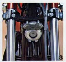
3. Hydraulic Disc steering damper for better handling on and off the road. It consists of an oil reservoir and a paddle in the steering column. When the handlebars are turned, the paddle works against the oil, damping the left and right travel. Ideal for dirt riding, since it prevents stones and ruts from radically deflecting the front wheel.
