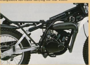
(Chassis: 2) The longer travel and the slower action of the monoshock suspension allows the rear wheel to follow the irregularities of the terrain, rather than bouncing over them. The ride is easier, progress faster, and maximum power is delivered to the ground. The rigid sub-frame keeps the wheel in alignment, minimizes weaving, and assists positive steering in the rough and on the road.
